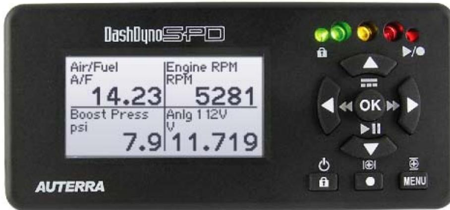
**Scan Tool / Performance Meter / Data Logger**
